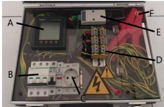
Gambar 1. Toolkit Alat Ukur Power Meter
